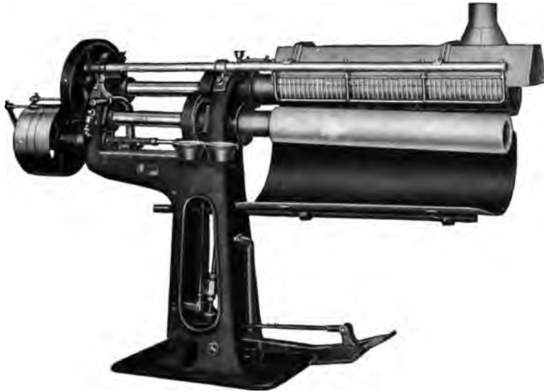
Fig. 1. Sleeve and Body Ironer equipped with Guard and Ventilating Hood.
